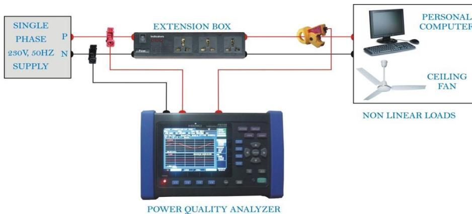
Fig. 4 Experimental Setup for personal computer and ceiling fan loads with PQA
