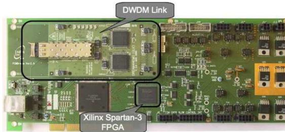
Fig. 1. Picture of the FCM board with the DWDM link plugged-in. The link interface and the test-bench controls are implemented by a software program running on an embedded microcontroller synthesized in the programmable logic.
