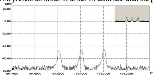
Fig. 5. Three-channels WDM spectrum with 100-GHz spacing.
