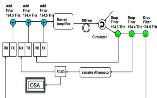
Fig. 4. Block diagram of the test-bench.
