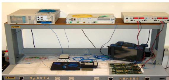
Fig. 3. Pictorial view of the experimental setup used to test the performance of the DWDM network
