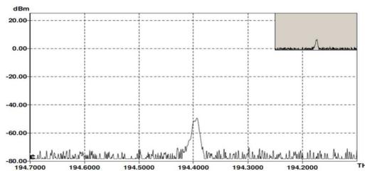
Fig. 6. WDM spectrum after Drop filtering.
