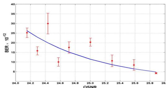
Fig. 9. Comparison between calculated BER and measured BER as a function of optical SNR (linear) for F440 transceiver.
