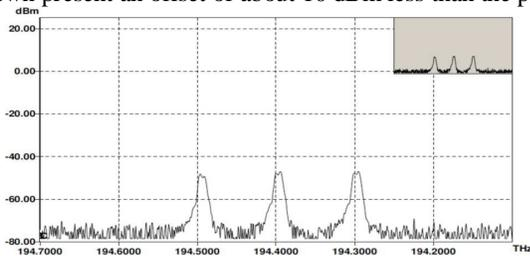
Fig. 5. Three-channels WDM spectrum with 100-GHz spacing.
