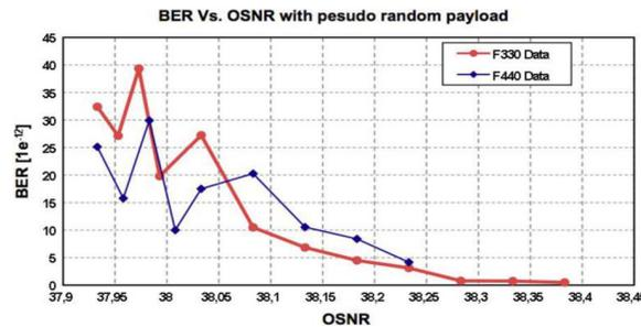
Fig. 8. Measured BER as a function of optical SNR at two different DWDM wavelengths.
