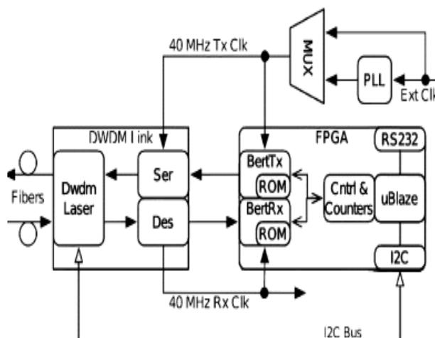
Fig. 2. Diagram of the FCM blocks, including the DWDM link and the FPGA functionalities.
