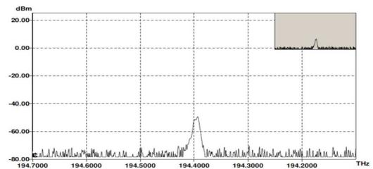
Fig. 6. WDM spectrum after Drop filtering.
