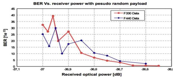
Fig. 7. Measured BER as a function of optical power at the receiver at two different DWDM wavelengths.
