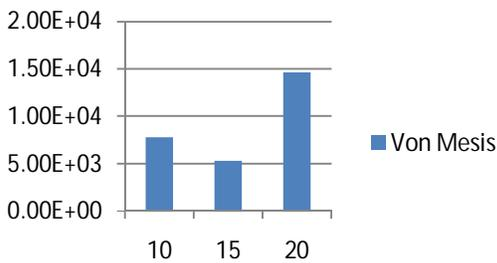
Fig 3: Stresses induced in canister with round bottom.
