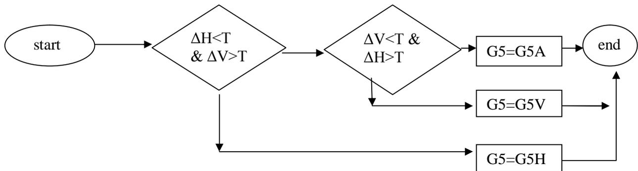
Fig.4. Flowchart for edge sensing method.
