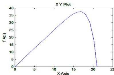
Figure.7 P-V Characteristics (Irradiation= $1000\text{W/m}^2$ , Temp= $25^\circ\text{C}$ ).
