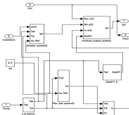
Figure6. The PV Cell Module Simulink Modeling.
