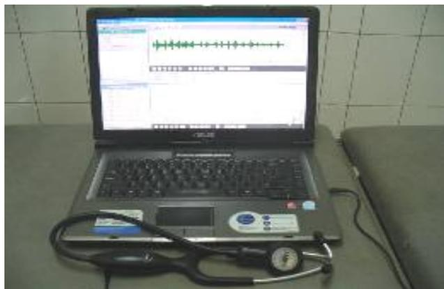
Fig. 2 Jables electronics stethoscope with laptop based phonocardiogram
