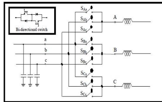
phase. Fig.2 shows the circuit scheme of three phase to three phase matrix converter. a b c input terminals and A B C output terminals
