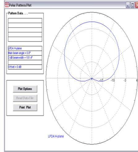
Figure 14: H-Plane pattern at 6 GHz
