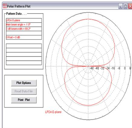
**Figure 11: E-Plane pattern at 0.5 GHz**
