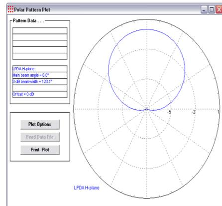
**Figure 12: H-Plane pattern at 0.5 GHz**
