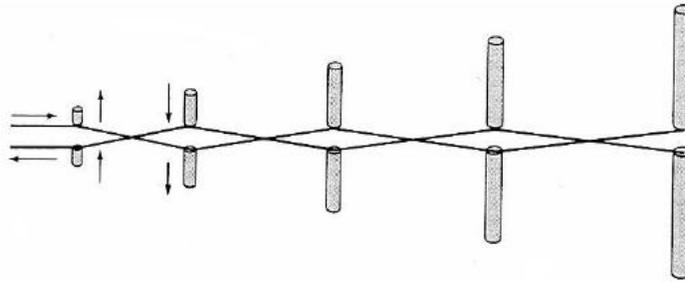
**Figure 4: Successful method of feeding the antenna**
