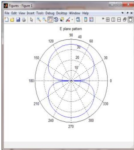
**Figure 9: E-Plane pattern at 6 GHz**
