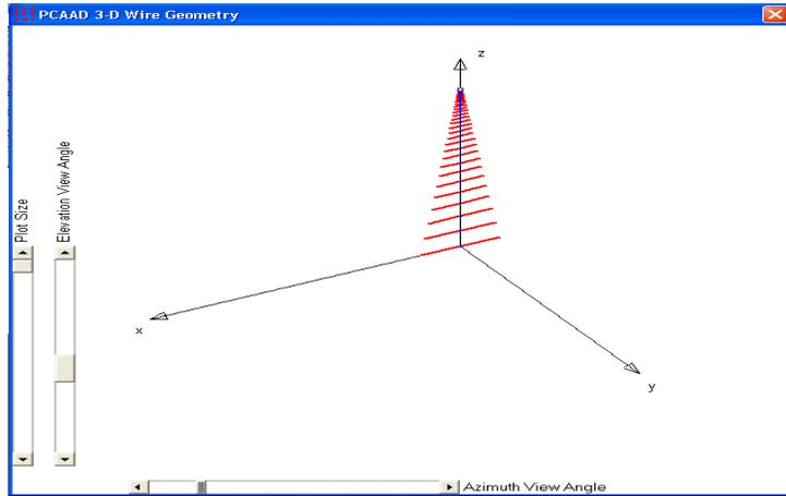
**Fig 6: The LPDA design using PCAAD Software**
