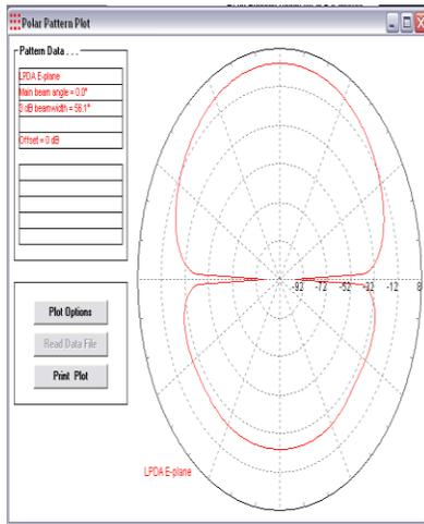
Figure 13: E-Plane pattern at 6 GHz
