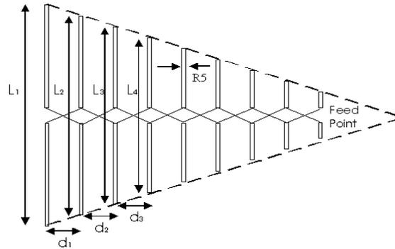
Figure 1: Schematic diagram of log-periodic dipole antenna
