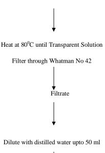
The concentration of respective metals is determined from the prepared solution on atomic absorption spectrophotometer model Chemito AA 203D.
