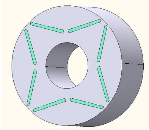
Fig. 2 IPM rotor
