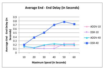
Figure 2: Average end-to-end delay vs. speed
