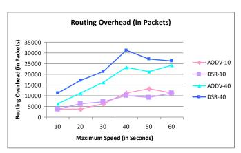
Figure 3: Routing overhead vs. speed
