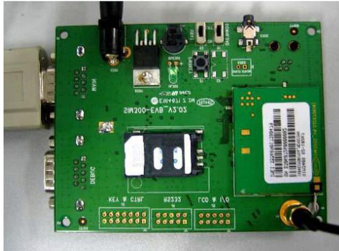
Figure 4. GSM MODULE
