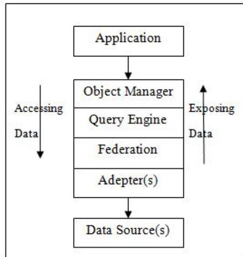
Figure1: ActiveRDF architecture
