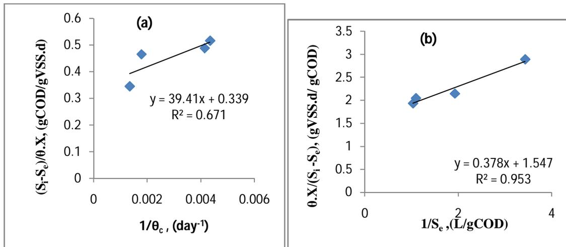
Fig 2. Diagram of determining synthetic coefficients of Y,  $K_d$ , K and  $K_s$  in monod model
