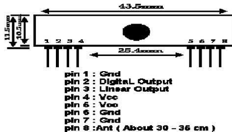
Figure 3.3: Pin out Diagram
