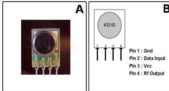
Figure 2.2: (A) TWS; (B) TWS-434 Pin Diagram
