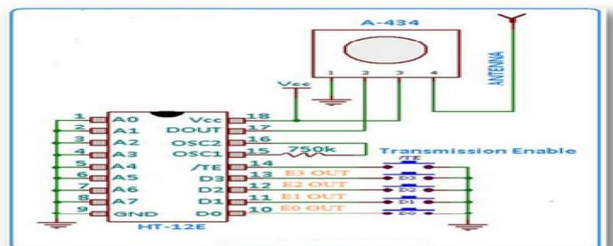
Figure 2.2: TWS-434 Transmitter Application Circuit
