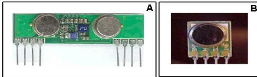
Figure 2:1 (A) Receiver Module; (B) Transmitter Module
