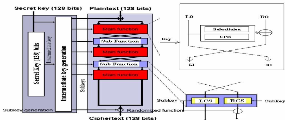
Fig. 1 Detailed Architecture of Encryption Process
