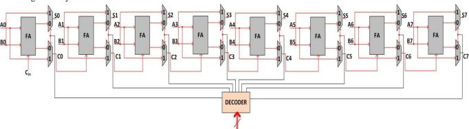
Figure 3: 8-bit reconfigurable RCA blocks.
