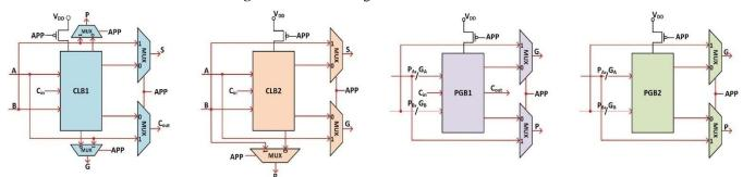
Figure 4: 1-bit dual-mode carry propagate generate blocks.
