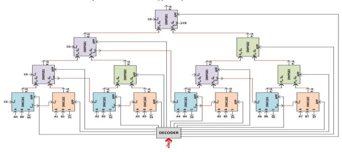
Figure 5: 8-bit reconfigurable CLA block.
