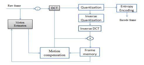
Figure 1: MPEG encoder block diagram.
