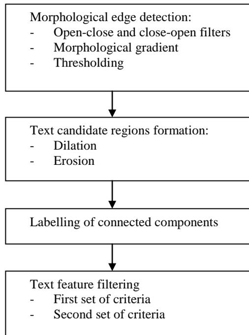
Fig. 1 Flow diagram of Text Detection algorithm
