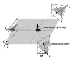
Fig. 1 Model of target localisation by multiple cameras
