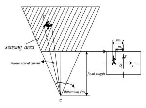
Fig. 2 Geometric model of target localization in the sensor image
