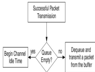
Fig 7.Successful Packet Transmission
