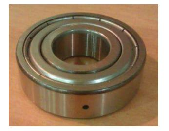
Fig. 3 Outer race fault
