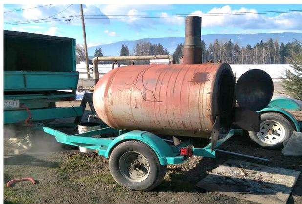
**Figure 3.** PRSI's mobile pyrolyzer unit.
