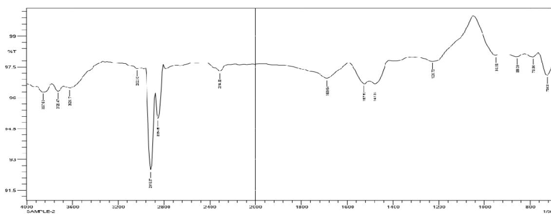
**Fig.5 FTIR spectra of low density polyethylene after 30 days incubation with Bacterial isolate 2**
