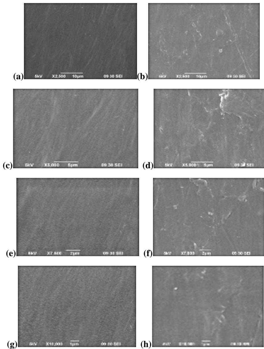
Fig .6 (a), (c), (e) and (g) untreated low density polyethylene at x2500, x5000, x7500 and x10000 respectively; (b), (d), (f) and (h) – low density polyethylene after 30 days incubation with Bacterial isolate 1 at x2500, x5000, x7500 and x10000 respectively.
