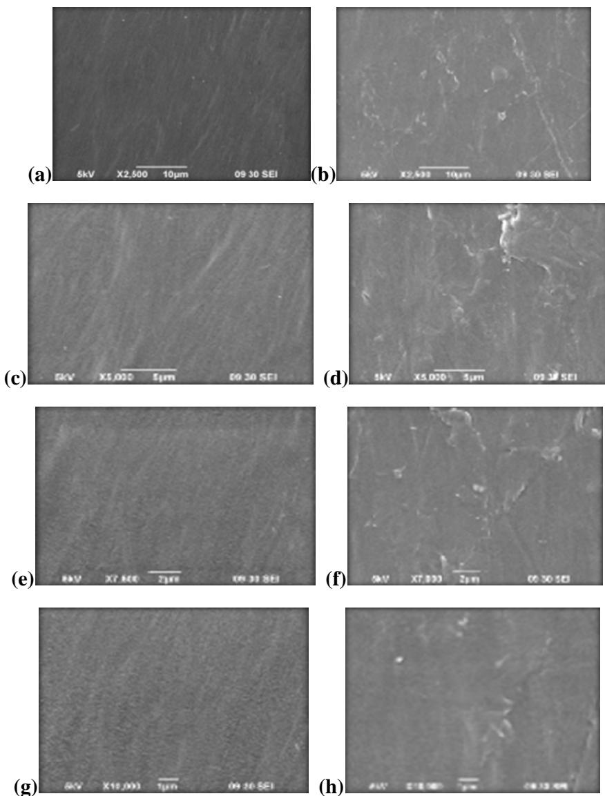
**Fig .6 (a), (c), (e) and (g) untreated low density polyethylene at x2500, x5000, x7500 and x10000 respectively; (b), (d), (f) and (h) – low density polyethylene after 30 days incubation with Bacterial isolate 1 at x2500, x5000, x7500 and x10000 respectively.**
