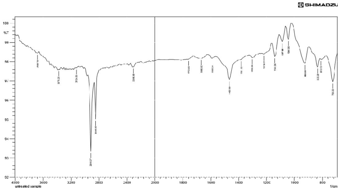
Fig.3 FTIR spectra of untreated low density polyethylene
