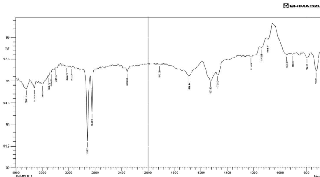
Fig.4 FTIR spectra of low density polyethylene after 30 days incubation with Bacterial isolate1
