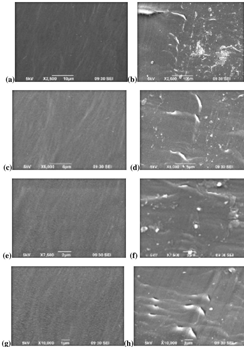
**Fig.7 (a), (c), (e) and (g) untreated low density polyethylene at x2500, x5000, x7500 and x10000 respectively; (b), (d), (f) and (h) – low density polyethylene after 30 days incubation with Bacterial isolate 2 at x2500, x5000, x7500 and x10000 respectively.**
