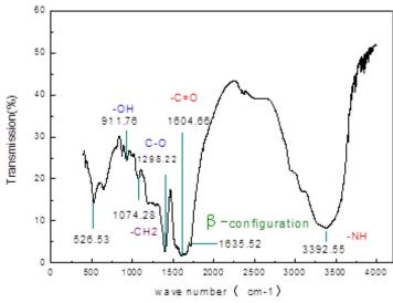
Figure 2. FTIR spectra of the copolymer PAC.
