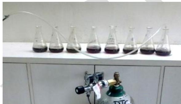
**Figure 1: Experimental setup with cylinder supplying carbon dioxide to the experiment flasks**
