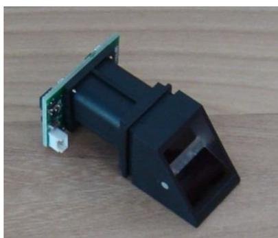
Fig. 4. R305 optical fingerprint scanner
