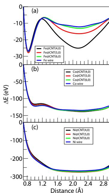
**Figure 1.** (Color online) Dependence of the energy of Fe, Co and Ni nanowires encapsulated by carbon nanotubes on the distance between the metallic atoms. For convenience, each dependence was shifted by its corresponding value when the distance was 0.70 Å.
