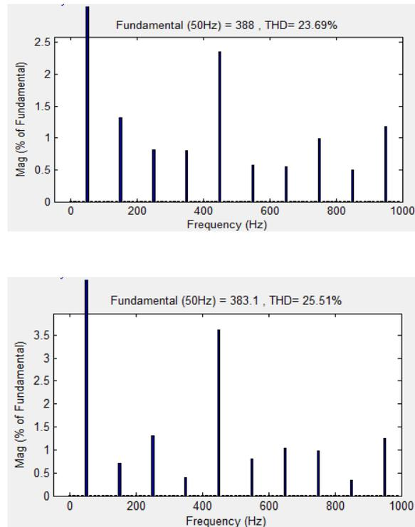
Figure 9. THD of three phase voltages
