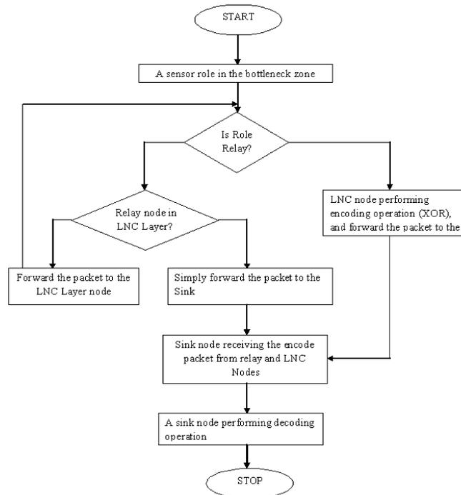
Fig 6: Flow chart of sensor node in bottleneck zone.
