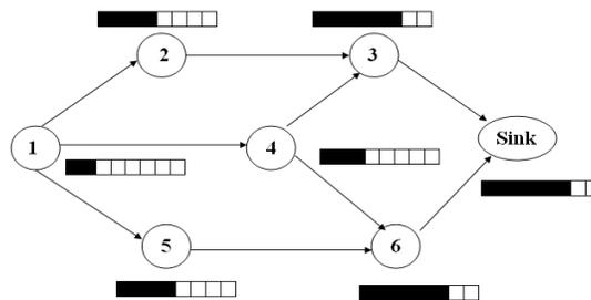
Fig. 3 Adaptive Duty Cycle in a typical WSN.
