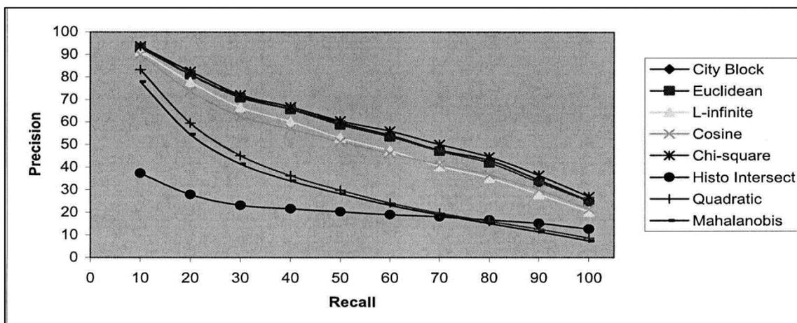
**Figure 5:** Performance of different distance measures on MPEG7 Set B [18].
