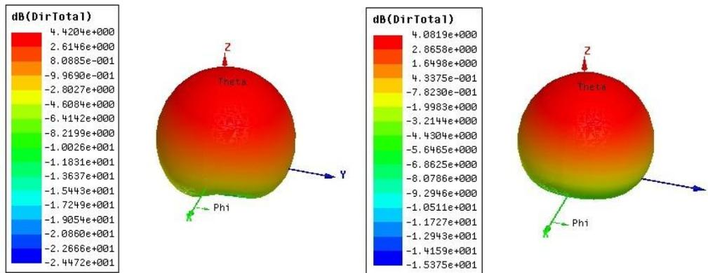
Fig 6.7: Gain of Psi shaped MSA Fig 6.8: Gain of Modified Psi shaped MSA
