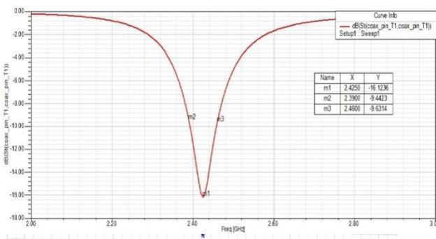
Fig 6.1:Return loss of Rectangular MSA
