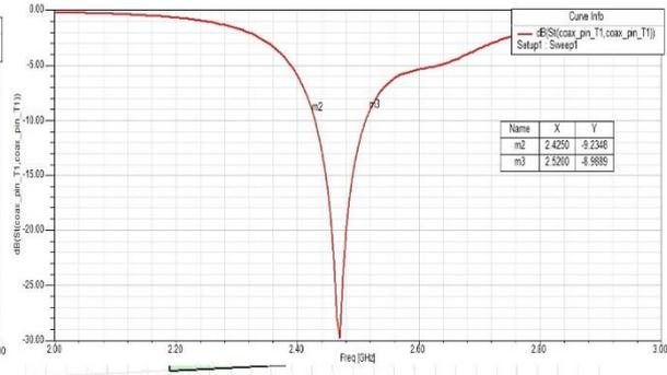
Fig 6.2: Return loss of E shaped MSA
