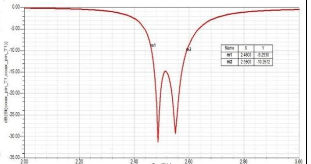
Fig 6.4: Return loss of modified shaped MSA
