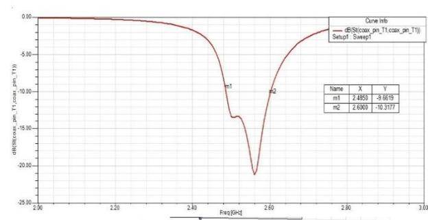
Fig 6.3:Return loss of Psi shaped MSA
