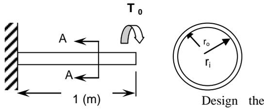
Section A-A, Outer radius -  $r_o$ , Inner radius -  $r_i$
