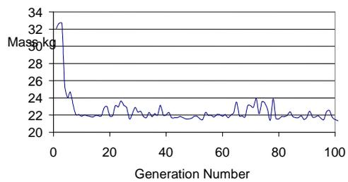
Fig (10) Minimum Objective Function Aluminium Alloy 24 ST4/L 0.75m
