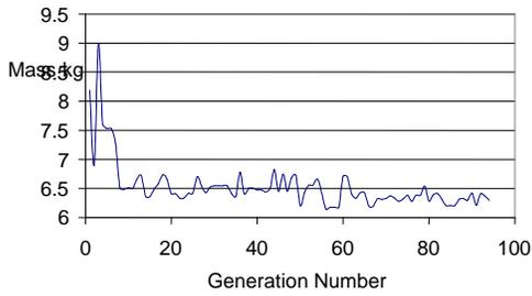
Fig (12) Minimum Objective Function Magnesium Alloy A261 /L 0.5 m
