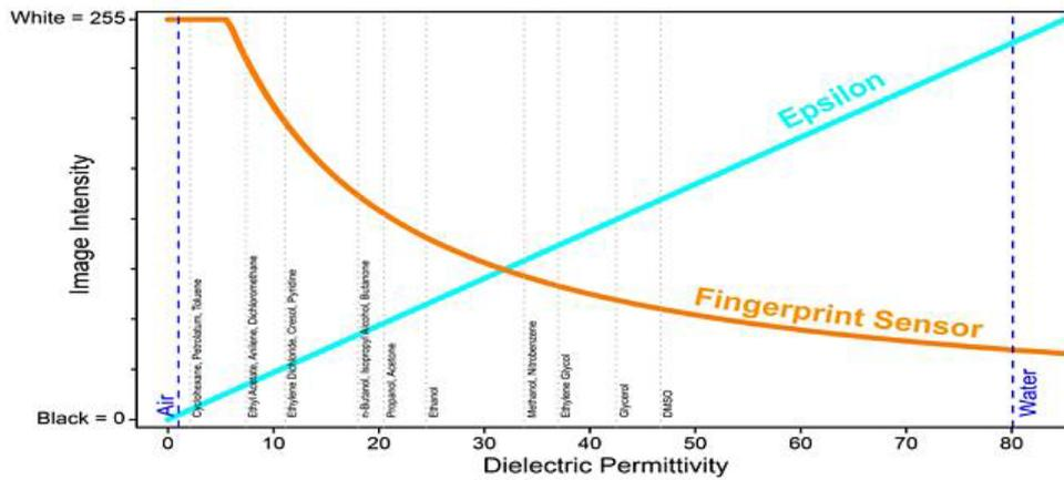
**Graph 6.** The calibration curve and linear response to dielectric permittivity.
