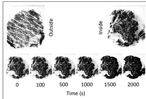
Capacitive contact images of the outside surface (top left), and the inside surface (top right) of in-vitro porcine tissue, and images of water penetration through the in-vitro porcine tissue (bottom) at different times (0-2,000 s)
