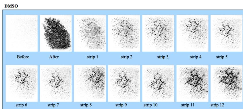
**Figure 7.** Fingerprint sensor images before and after DMSO application and subsequently during tape stripping.
