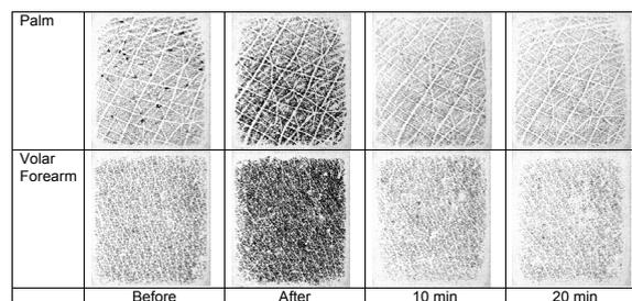
**Figure 4.** Capacitive images of two different skin sites, palm and volar forearm, before and after a 5 min wet tissue patch hydration.
