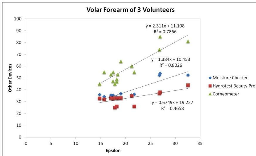
**Graph 7.** The comparison results of Epsilon and Moisture Checker, Hydrotect and Corneometer.
