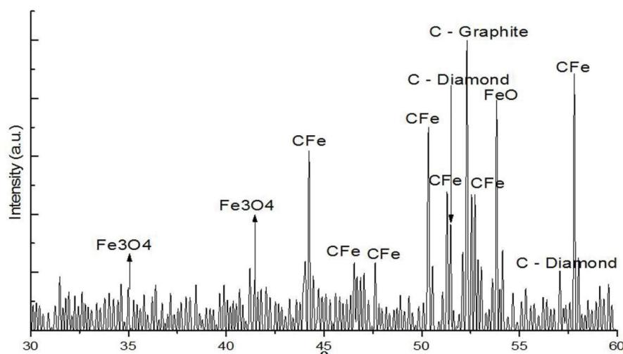
**Figure 4:** X-ray diffraction patterns for DLC film deposited on the steel AISI D2 surface with graphite cage; (B) crystallographic data for iron carbide  $\text{Fe}_3\text{C}$ .
