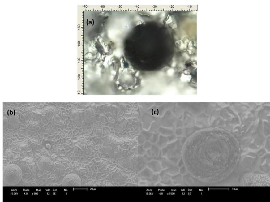
**Figure 3:** Analysis of (a) optical and (b and c) scanning electron microscopy of the DLC coating.
