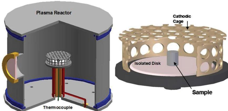
**Figure 1:** Configuration of the cage used and the way it was placed in the reactor.
