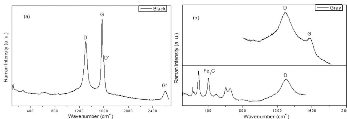
**Figure 5:** Micro-Raman spectroscopy analysis of the dark and gray regions of the film deposited in D2 steel, using a laser of 785 nm.
