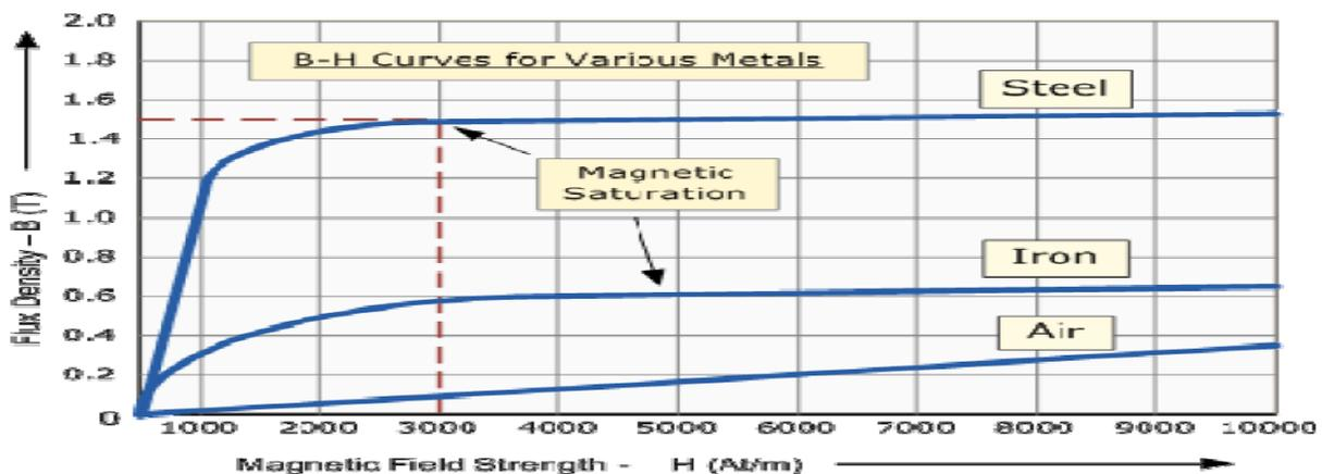
Figure 3: B-H Curve for magnetic materials
