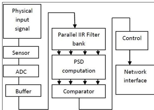
Fig. 5. WINS digital signal processing.
