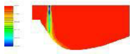
FIG.16: VELOCITY IN THE Y-DIRECTION (SYMMETRY)
