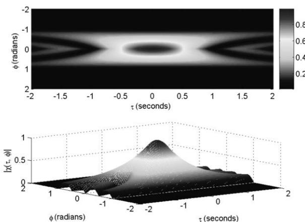
**Figure 1: Lateral information function plots for a single frequency feature. The delay unit ( $\tau$ ) is seconds, the robust feature unit ( $\varphi$ ) is radians and the absolute value of the lateral information function scale is linear. The feature duration is two dimensional.**
