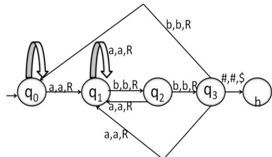
Figure 5: Turing machine for L
