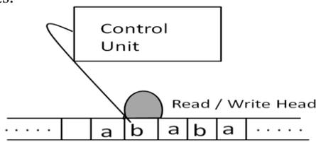
Figure 2: Turing Machine Model
