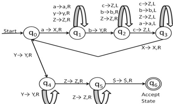
Figure 4: Transition diagram for  $L = \{a^n b^n c^n \mid n \geq 0\}$
