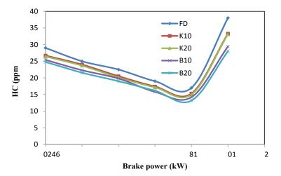
Figure 7: Variation of HC emission with brake power.
