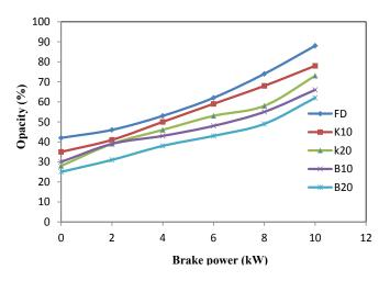
Figure 9: Variation of smoke opacity with brake power.
