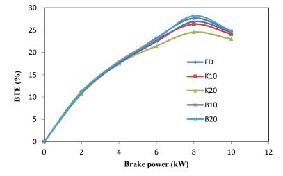
Figure 4: Variation of BTE with brake power.
