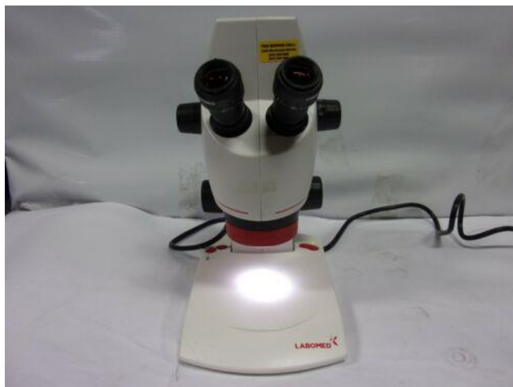
Figure 1. Stereomicroscope imaging of the vertical dye penetration (Labo Med CMZ4, India).
