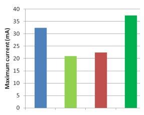
Vulcan XC 72 RP 20 NORIT YP 50F Fig 3 Characteristics of maximum value of current for different types of carbon materials
