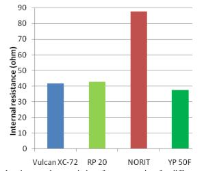
Fig 4: Internal resistance characteristics of supercapacitor for different supercapacitor
