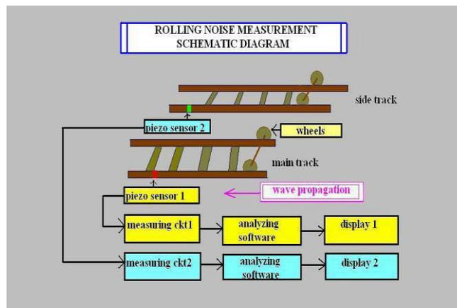
Fig. 4 Measurement of rolling noise on both tracks
