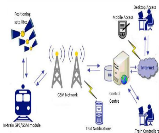
Fig. 1 GPS/GSM architecture
