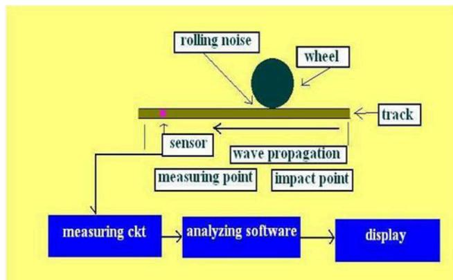
Fig.3 Measurement of rolling noise
