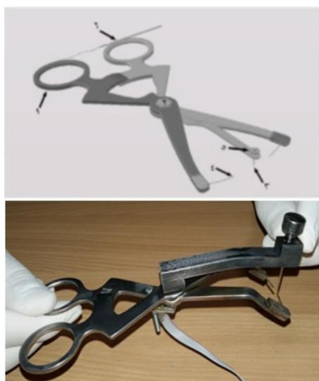
**Figure 3.** Mechanical part of the gauge includes (I) handles adjusting the horizontal pins, (II) location of magnet and IC magnetic sensor, (III) vertical pin, (IV) horizontal pin, (V) screw to adjust the vertical pin and (VI) wire connecting the magnetic sensor to the main circuit.
