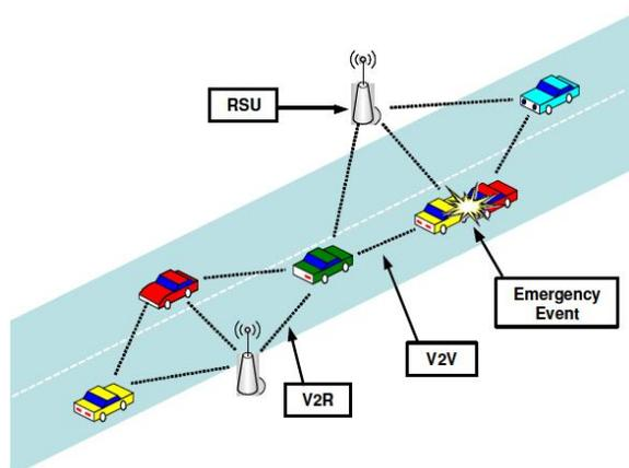
Fig 1: Example of a VANET [14].
