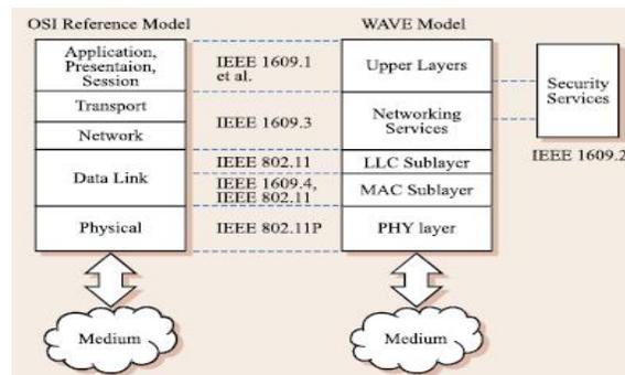
Fig 2: WAVE Model and OSI reference model [11].
