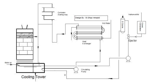
Figure-1.Block diagram for ozone treatment (pilot plant) of cooling tower water
