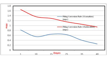
Figure-5: Pitting corrosion plot during ozone disinfection and chlorination
