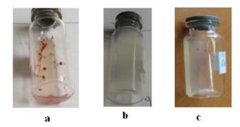
Figure-8: Figures of TBC test, in the conditions of a. lack of disinfection b. ozone disinfection in 0.1 mg/lit concentration, c. chorine in concentration lower than 0.2 mg/l that was calculated according test kit method with the standard B9215
