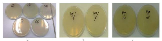
Figure 7-a- TBC test is illustrated before disinfection that was calculated according to ASTM D5465 b-TBC test is illustrated, in disinfection time with chlorine 0.5 mg/lit concentration c in disinfection time with ozone 0.1 mg/lit concentration that was calculated according to ASTM D5465.
