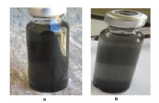
Figure-9: SRB test is illustrated before disinfection b- SRB test is illustrated, chorine in concentration lower than 0.2 mg/lit.
