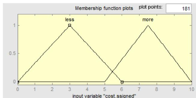
Fig 12: Membership function for cost assigned
