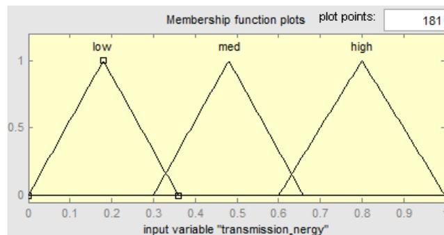
Figure 8: Membership function for Transmission energy
