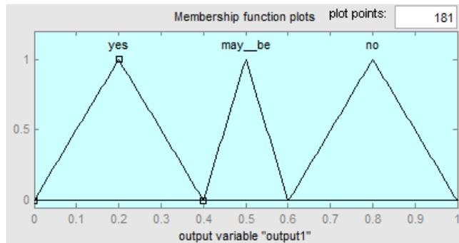
Fig 13: Membership function for output
