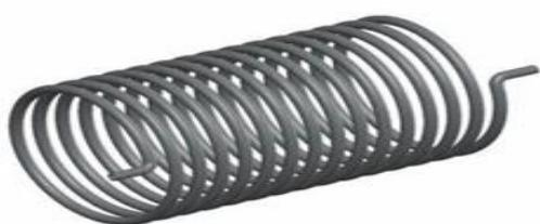
**Figure 3.2.** Inside view of tube in tube reactor.
