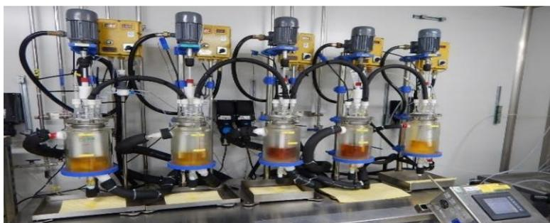
Agitation reactors are based on the principle of continuous stirred tank reactors. It features a reaction block which is mounted on the agitator [15]. The agitation reactor utilizes freely moving agitator within the reactor block. The
