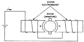
Figure 6: DC motor with electromagnet as stator
