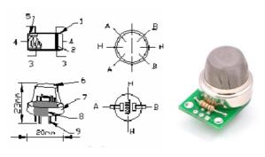
Figure 4: The structure and configuration of MQ6 gas sensor
