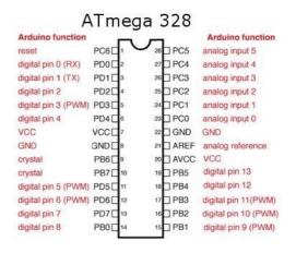
Figure 3: ATmega328 p microcontroller
