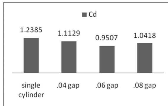
Fig.5 Net effect of Cd on both the cylinders
